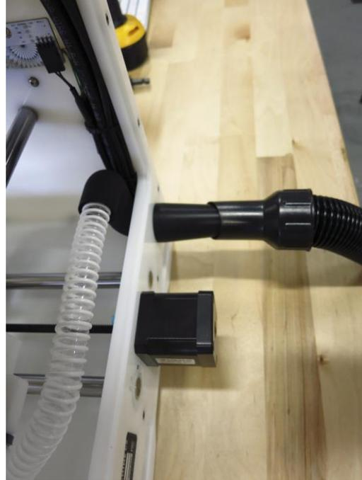
**IMPORTANT:** The vertical lines of the Vacuum Port Fitting or Double Elbow should be perpendicular to the ground when the system is in place. If it is rotated, your T-Slot Bed will collide and be unable to successfully run. If your hole is centered and the Vacuum Port Fitting is arranged correctly you should not have clearance issues.
