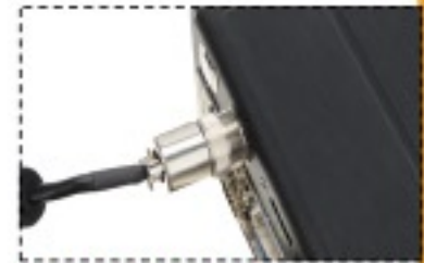
Secure and keyed DC-in connector
